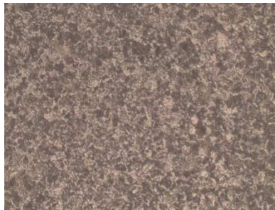
Figure 8: Microstructure of Cyclic Heat Treated Specimen, 10 Cycles (200×)
