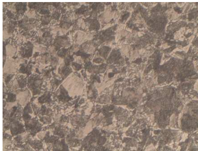
Figure 4: Microstructure of Cyclic Heat Treated Specimen, 2 Cycles (500×)
