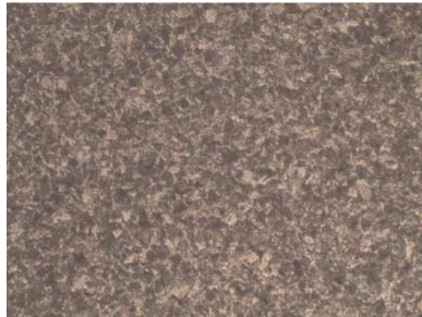
Figure 7: Microstructure of Cyclic Heat Treated Specimen, 8 Cycles (200×)
