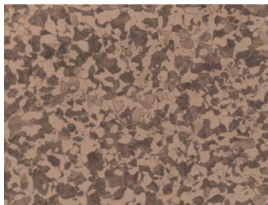
Figure 1: Microstructure of As-Received C45 Steel Specimen (200 \times )
